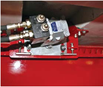
Air operated locking system on sliding A-trailer from Freighter MaxiCUBE Advance (on left), cable lock down on Freighter EzyLiner (above), stylish filler panels smooth airflow (on right).
