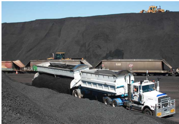
ABOVE: It is important to keep the payload central in the Side Tippers during actual tipping to ensure the load weight remains central and doesn't slide to the side when tipping.
