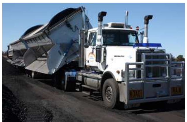
ABOVE: It is important to keep the payload central in the Side Tippers during actual tipping to ensure the load weight remains central and doesn't slide to the side when tipping.
